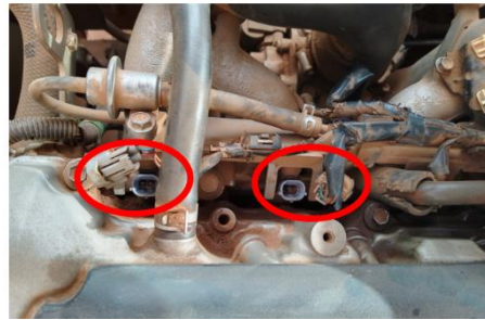
Figure 5: View of the engine with 2 injectors disconnected
