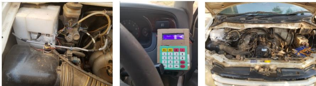
Figure 11: Captures of the password-based immobilizer produced and mounted on a Toyota NOAH vehicle
